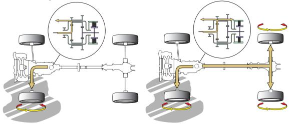
The hydraulic system of the VTD AWD is basically the same as that of the MP-T AWD, consist of a transfer duty solenoid, transfer control valve, and LSD clutch. The transfer duty solenoid is operated by the duty signal sent from the TCM.
