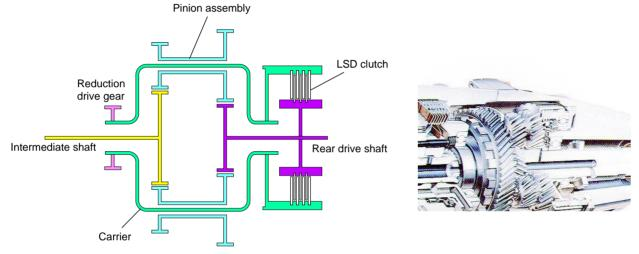
During normal driving, the LSD clutch is in released position, allowing the center differential to compensate for the rotational differences between the front and rear axles and to distribute the driving force transmitted from the engine to the front and rear axles in 45: 55 proportions.
