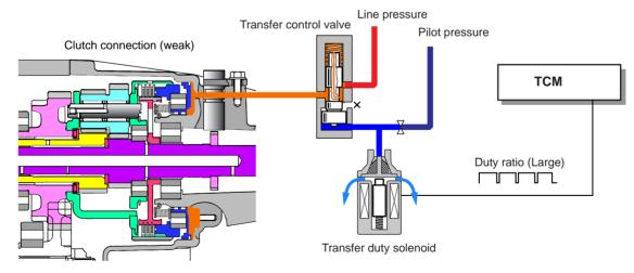
The relationship between the duty ratio of the driving signal from TCM and the condition of the LSD clutch engagement is shown in the table below.
