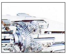
A center differential made up of composite planetary gear sets is installed among the intermediate shaft, which is the output shaft of the transmission, and the rear drive shaft connected to the propeller shaft. Also, at the rear end of the center differential, a multi-plate clutch (LSD clutch) which limits the operation of the center differential is installed.
