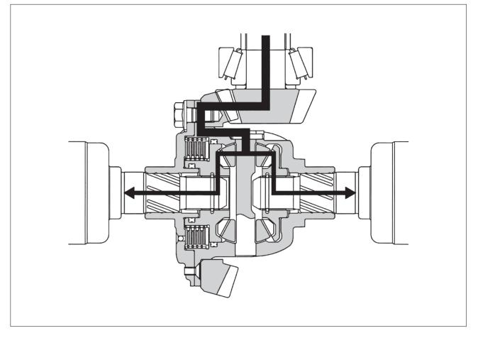
Under normal driving conditions, when the left and right wheels are turning at the same speed, the side gear rotates together with the differential case and the driving force is evenly distributed to the left and right sides, as with a normal differential.
