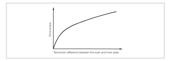
Therefore when the car is turning at the corner, viscous coupling does not produce so much torque due to small speed difference between right wheel and left wheel and when one wheel is slipping, large torque is produced due to large speed difference.
