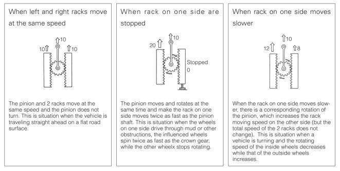
These figures explain the working principle of the differential in terms of 2 racks (equivalent to side gears) and a pinion. Three cases are described: when the 2 racks move at the same speed; when one rack is stopped; and when one rack moves at a reduced speed of 8, with the pinion moving speed (equivalent to crown gear rotating speed) assumed to be 10.
