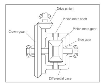
The rotation of the drive pinion is transmitted to the crown gear, which is geared to the drive pinion, and it is then transmitted from the differential case to the pinion mate shaft, thereby turning the side gears via the pinion mate gear. Since there is no difference in the rotating speed of the left and right wheels, the pinion mate gear revolves with its shaft but does not turn around the axis of the shaft, and the left and right side driving force ratio is 50:50.
