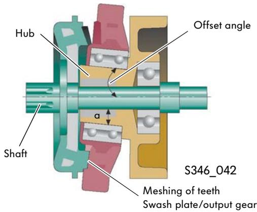
The shaft is securely joined to the output gear. The large gear wheel is mounted on this shaft. The swash plate is pushed onto the hub of the large gear wheel. This hub is designed so as to allow an offset angle between the hub and the shaft. This offset angle triggers the roll motion of the swash plate.
