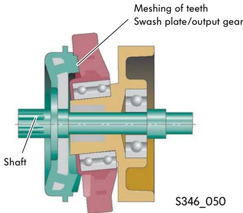
During one rotation of the large gear wheel, two teeth of the swash plate and output gear respectively will always engage. This means that engagement always occurs at the position where the hub of the large gear wheel has the lowest material thickness (a).
