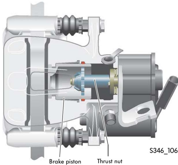
Brake pad replacement is carried out with the electromechanical parking brake not applied. With the aid of vehicle diagnosis, testing and information system VAS 5051, the electro-mechanical parking brake is opened fully, whereby the thrust nut is moved back completely on the spindle. Resetting of the electromechanical parking brake is again carried out with vehicle diagnosis, testing and information system VAS 5051. The new position of the brake pads is matched automatically.
