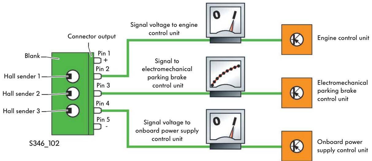
Hall sender 1 is a digital sender. It sends its voltage signal to the engine control unit. The signal results in the cruise control system being switched off.
