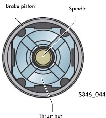
The thrust nut has longitudinal mountings in the brake piston. This means that it is restricted to axial movement. The inner shape of the brake piston and the shape of the thrust nut prevent the nut from twisting.
