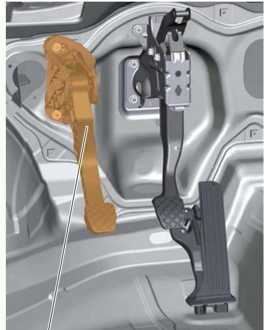
Clutch pedal with clutch position sender
