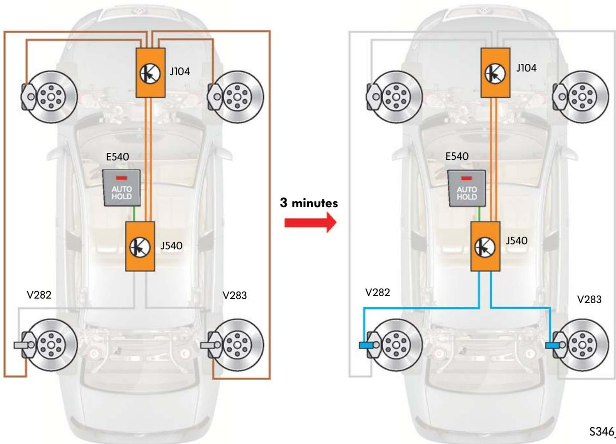
1. The AUTOHOLD function is active. The vehicle is stationary and is held in position by the 4 wheel brakes. The pressure required for this is calculated and set depending on the gradient by the ABS control unit.
