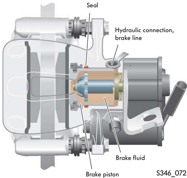
In the event of a dynamic emergency stop (pressing of electromechanical parking brake button while the vehicle is in motion), the pressure of the brake fluid is increased via the brake line. This pressure causes the brake piston to press against the brake pads. The brake pads press against the brake disc. When this happens, the seal is pressed out of shape towards the brake pads.
