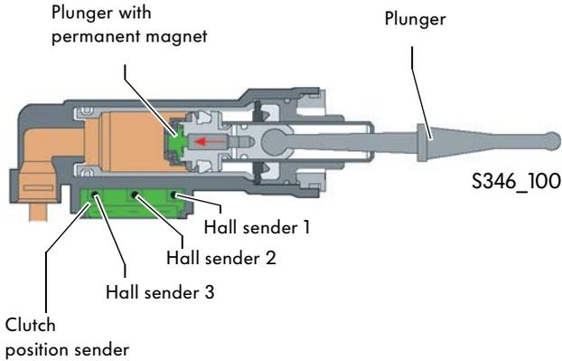
When the clutch pedal is pressed, the push rod and plunger are pushed in direction of the clutch position sender. At the front end of the piston is a permanent magnet. Integrated in the clutch position sender are three Hall senders on a blank.
