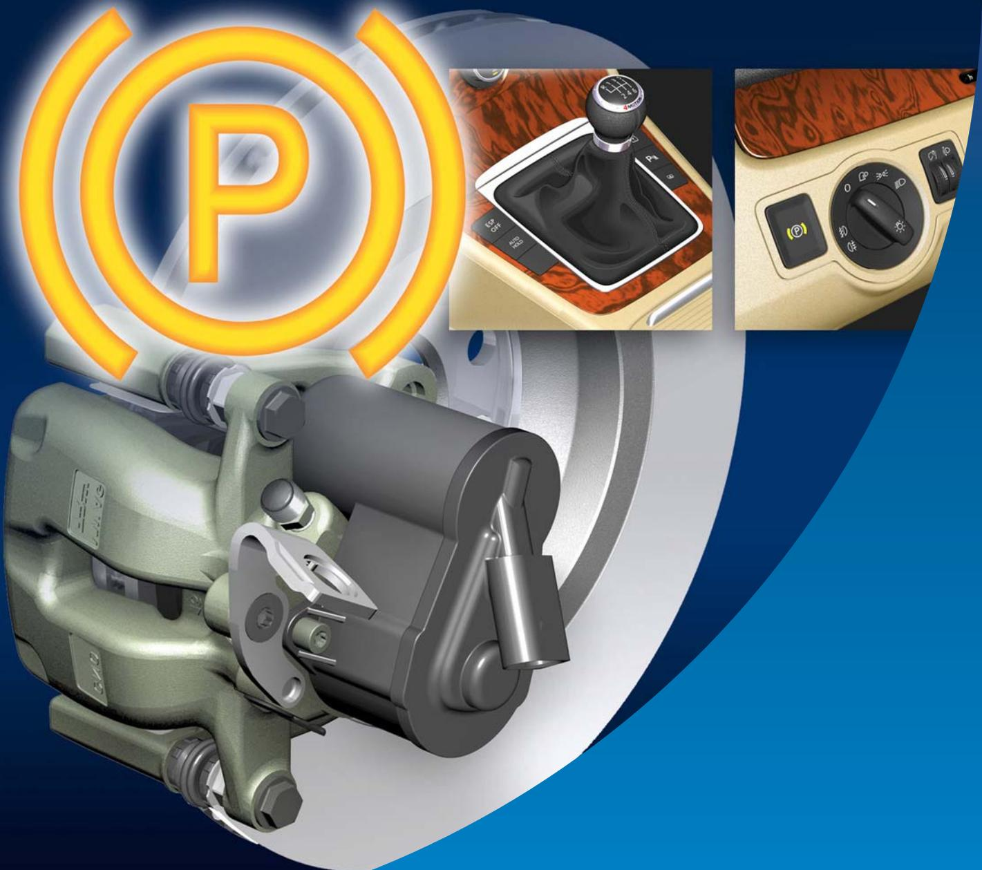
To make absolutely sure that the vehicle could not roll away when parked up, the driver had to pull up sharply on the handbrake lever until now or step on an additional parking brake pedal in the footwell. In the future, all that will be required is a quick press of a switch in the instrument panel – thanks to the electromechanical parking brake in the new Passat replacing the conventional, manual parking brake.
