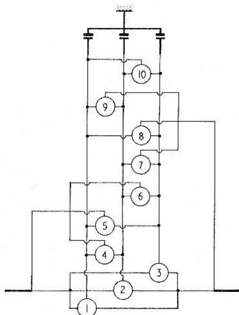
Fig. 13. Complete network for 3-speed gearbox design
