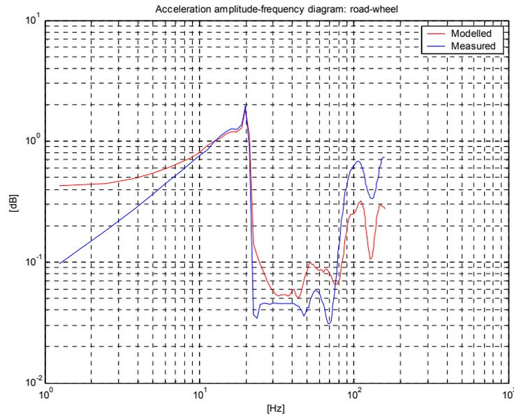
Figure 12: Road-wheel acceleration frequency diagram
