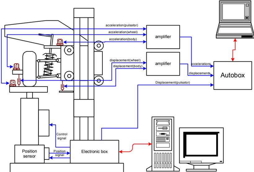
Figure 3: Measuring system
