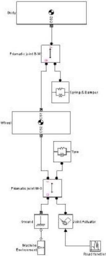
Figure 9: The Simmechanics model
