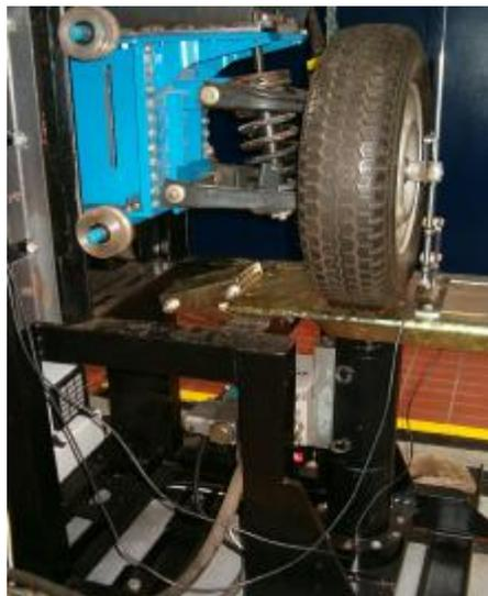
Figure 2: The hydraulic pulsator
